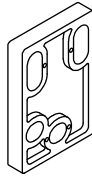
spacer plate for face fixture 100 × 150 × 20 mm N.B! Stack to a max. height of 200 mm
